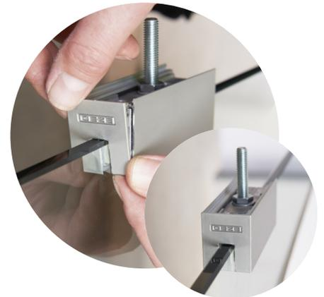
9 Select the right end cap to suit the glass thickness. Cut the section out to enable the cap to slide over the glass and clip onto the end of the clamp.
